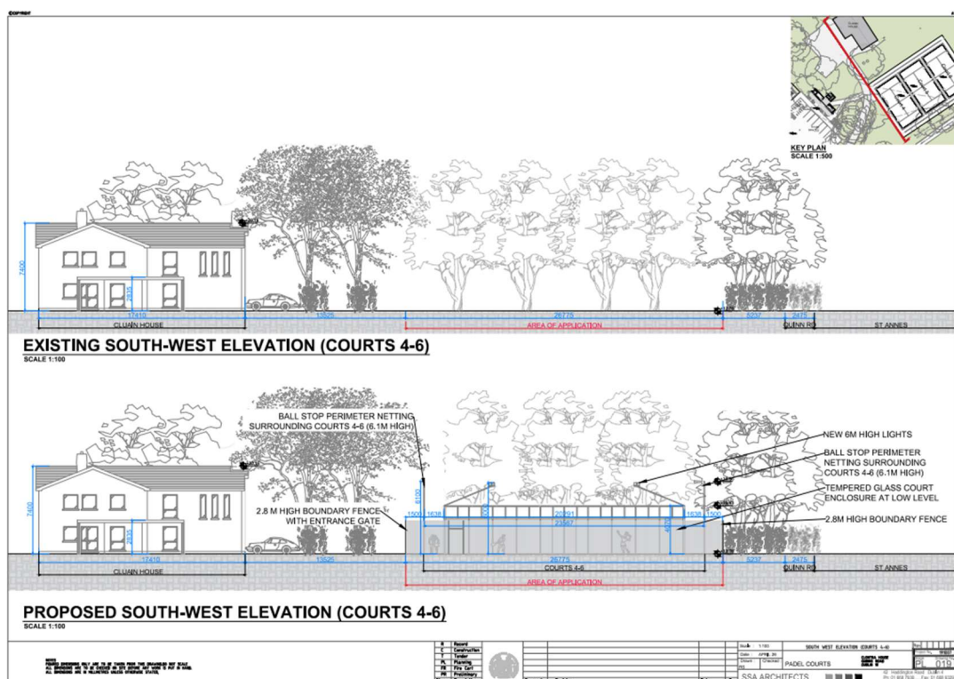
Fig. 18: Existing and Proposed South-West Elevation for Courts 4-6
